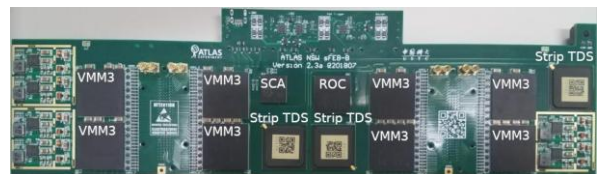
Photo of sFEB, Frontend and backend electronics for the New Small Wheel Upgrade of the ATLAS muon spectrometer, TWEPP 2018, edited
