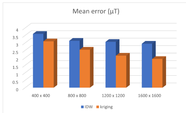
Figure 5.4 Comparison of average error for the geomagnetic field obtained via IDW and Kriging
