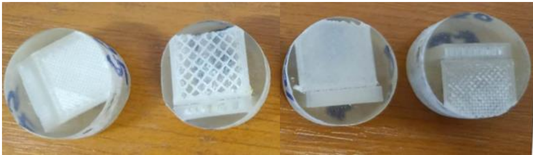
Fig. 12. Samples prepared for quality evaluation of 3D FFF-printed surfaces with glass fiber composite filament (Nicolau et al. , 2022)
