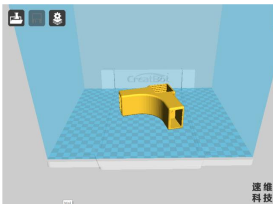
Fig.10. Position 1 (horizontal) of 3D printing of the connector.
