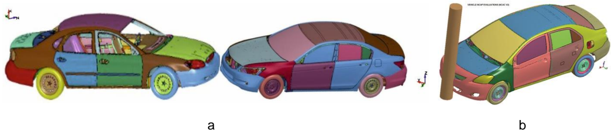
Fig. 4.1 Frontal collision: a) car-car; and b) automobile-cylindrical vertical obstacle
