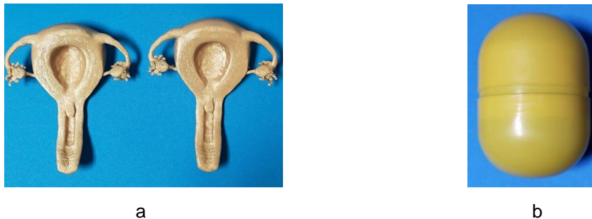
Fig. 6.19 Tested uterus models: a - different materials and b - cylindrical shape
