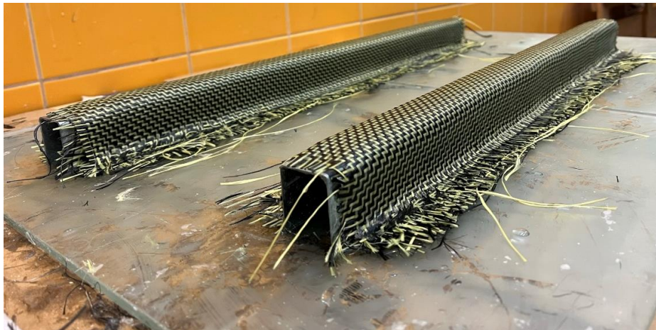
Figure 7.1. U-type profile made of hybrid composite material obtained by manual layering technology ("lay-up" technology).
