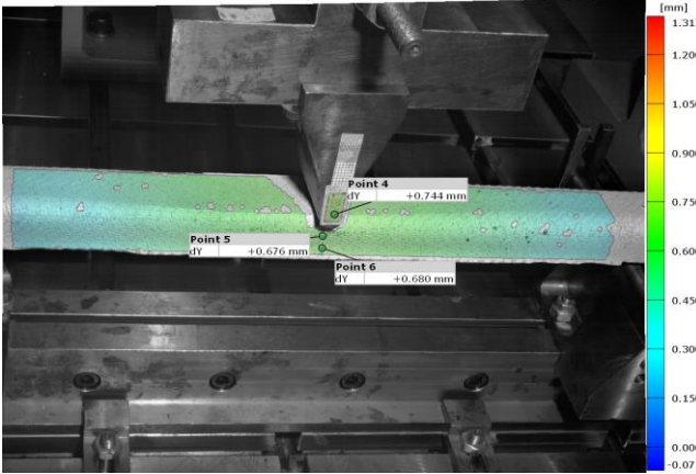
(k) Displacement v = 0,676 mm for F = 659,01 N
