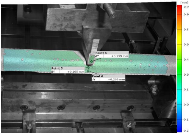
(c) Displacement v = 0,265 mm for F = 246,17 N
