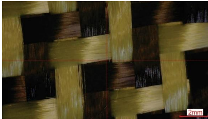
Figure 5.1. Photo of the SIGRATEX H W215-TW2/2 twill woven carbon-aramid fabric used to reinforce the laminated composite material tested [60].
