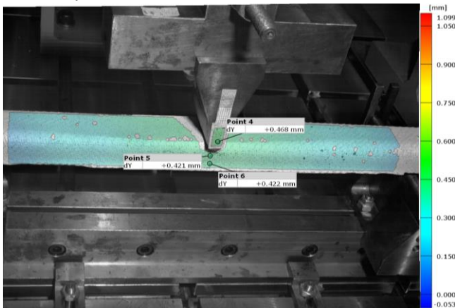
(f) Displacement v = 0,421 mm for F = 403,38 N
