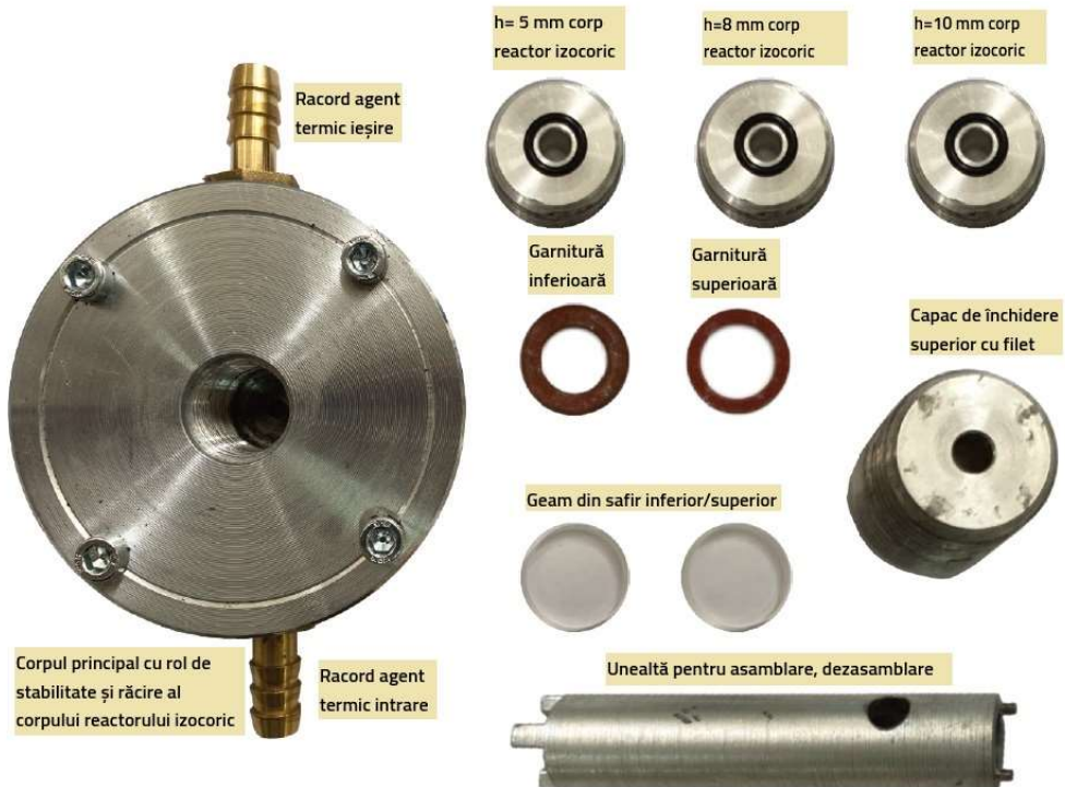
Figure 24 - Isochoric visualization device – the real model, with its functional components disassembled
