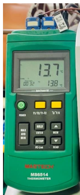
Termocuple conectate la termometru digital Mastech MS6514
