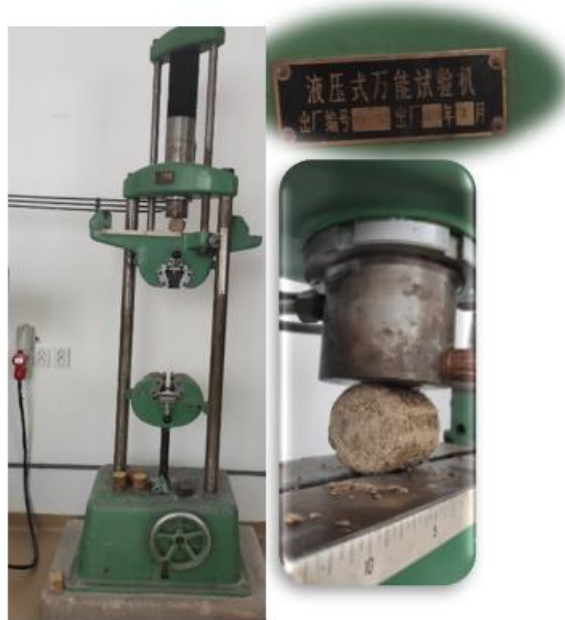
Figura 3.10: The machine for determining compressive strength (made in China/of Chinese production)
