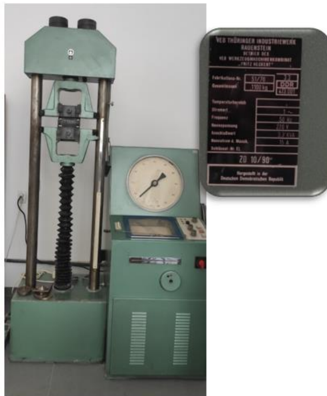
Figure 3.14. The machine used for determining splitting strength (made in Germany)
