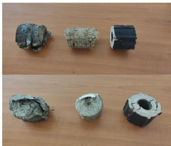
Figure 3.13: Lignocellulosic briquettes obtained during the determination of compressive strength
