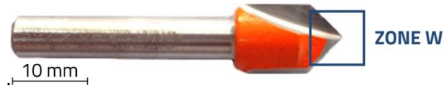
Fig. 4.7. Zone W of investigation the wear of the tool cutting edge (Lungu et al. , 2021c).
