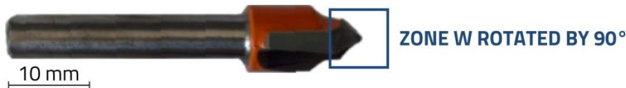
Fig. 4.8. Zone W rotated by 90° of investigation the wear of the tool cutting edge (Lungu et al. , 2021c).
