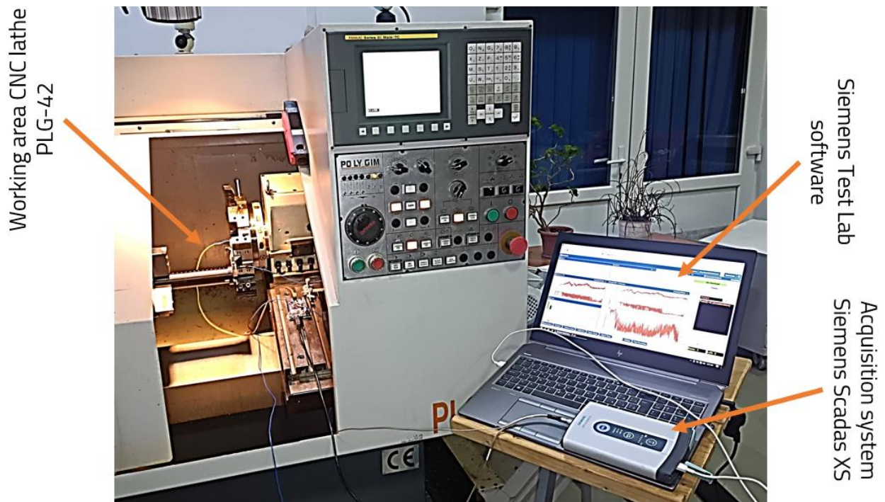
Fig. 4.86 Generic setup for measuring tool-tip inertances on the PO PY GIM PLG-42 CNC lathe
