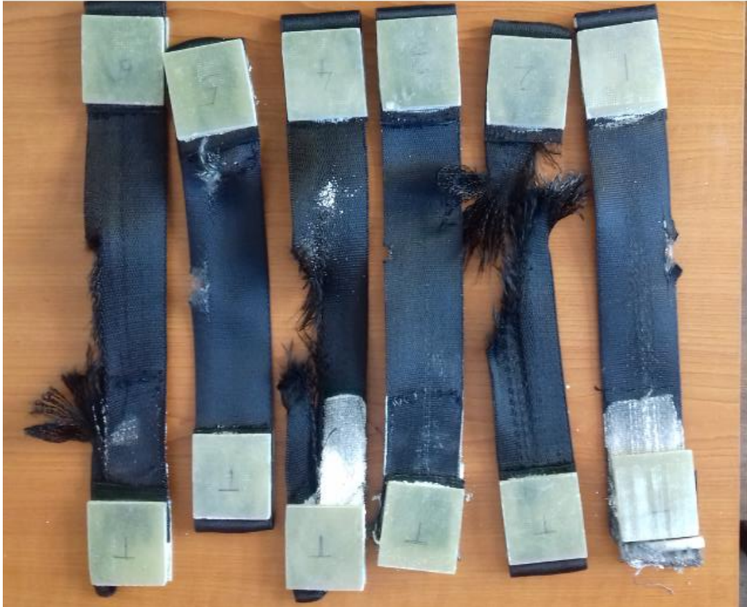
Figure 5.22 Samples after testing for cut webbing
