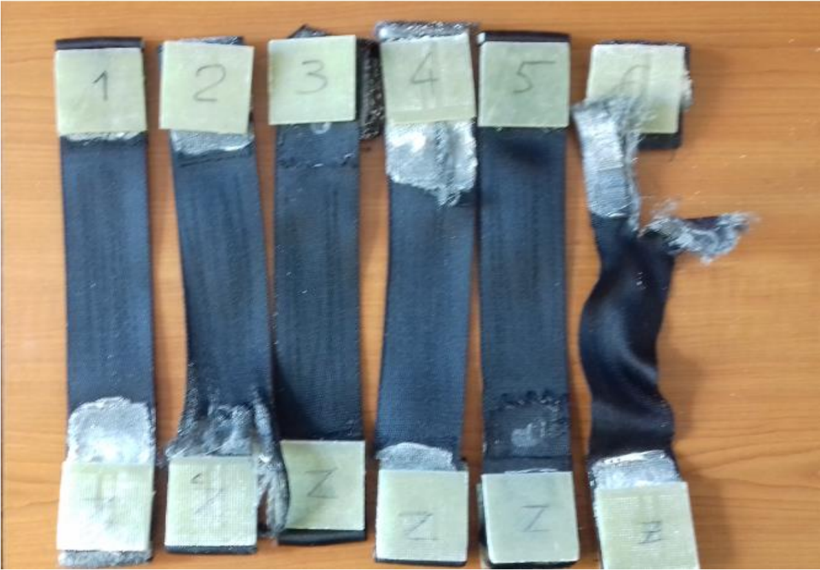
Figure 5.31. Samples after testing for scratched webbing
