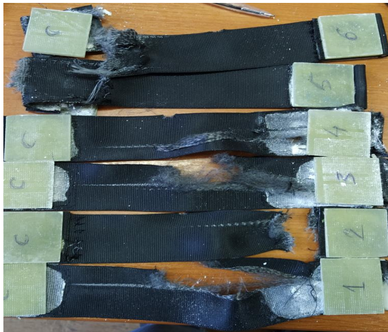
Figure 5.14 Burnt webbing samples after testing
