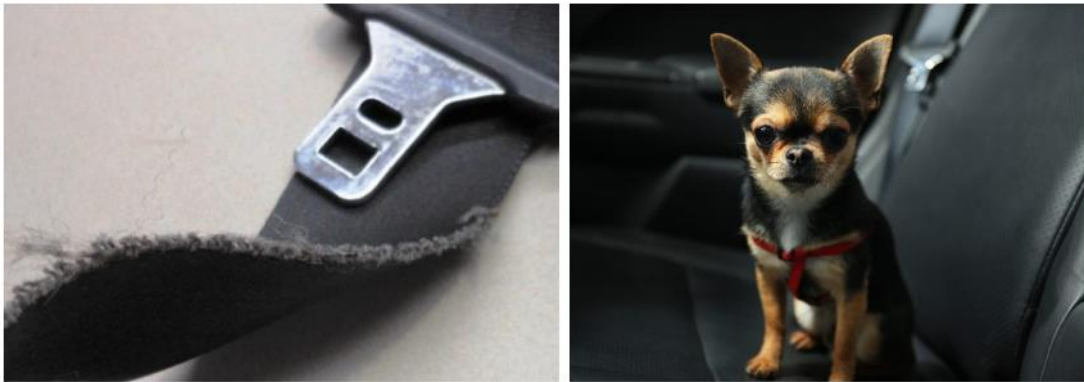
Figure 1.16. Webbing deteriorated after incorrect animal transportation
