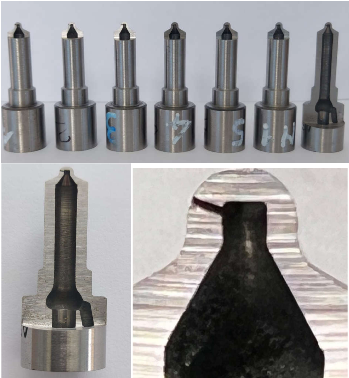
Figure 7.22. Sectional injection sprayers in the area of the spray channel
