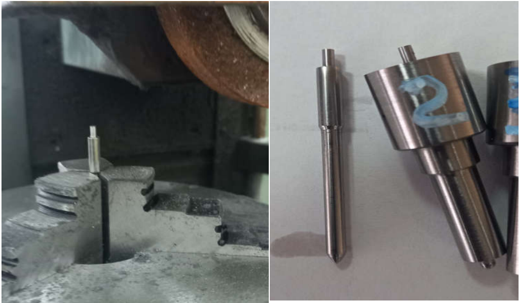
Figure 7.5. Device for fixing the spray needle on the UMG Cugir grinding machine
