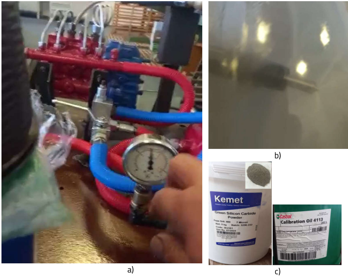
Figure 7.1. The processing of injection sprayers: a) - functional presentation; b) - presentation of the spraying of the fuel jet in the collection tank; c) - presentation of SiC micropowder - F 800, and calibration oil 4113 used in processing
