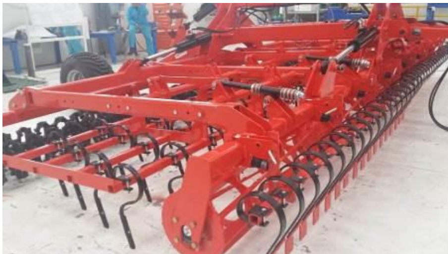
Fig. 2.4 Vibrocombinator echipat cu organe active de tip GAMA Fig. 2.4 Vibrocombinator equipped with GAMA type active organs
