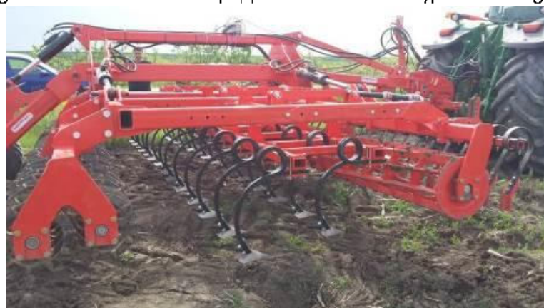
Fig. 2.6 Vibrocombinator echipat cu organe active de tip DELTA 2 Fig. 2.6 Vibrocombinator equipped with DELTA 2 type active organs
