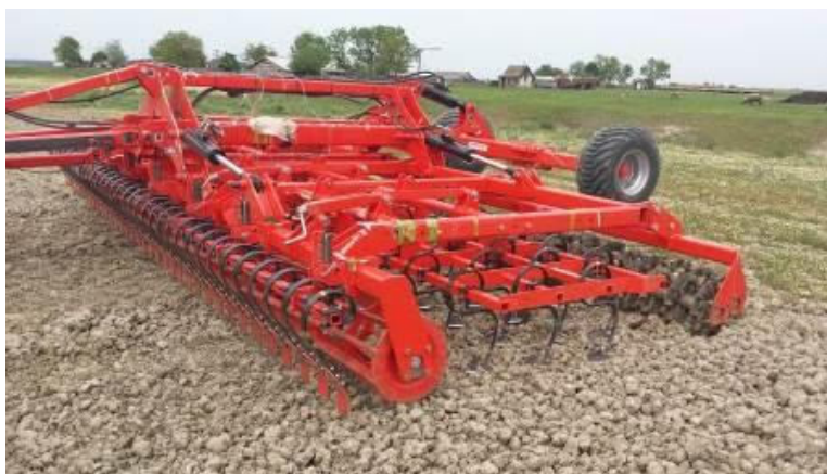
Fig. 2.5 Vibrocombinator echipat cu organe active de tip DELTA 1 Fig. 2.5 Vibrocombinator equipped with DELTA 1 type active organs
