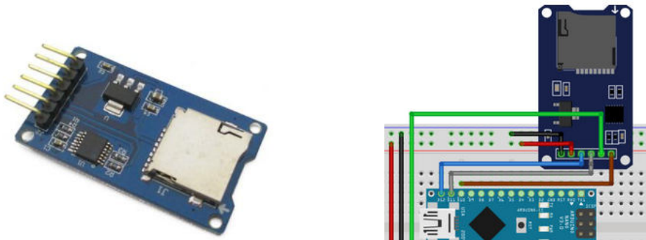
Figure 6.6 SD memory card adapter (a) mounting kit, (b) connection diagram
