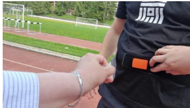
Fig. 111 – Placement of the Xsens sensor on the subject
