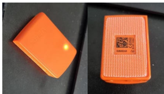
Fig. 109 – Xsens sensor used for parameter records of the 6 subjects
