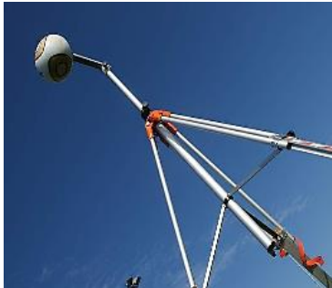
Fig.4.47. Vertical Deltec Ball Rebound Tester ( http://www.deltecequipment.com/wp/producten/pro-line-apparatuur/vertical-ball-rebound-tester/ )
