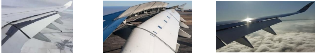
Fig. 1.2 Flaps simplu element sau monobloc Airbus 340, 380, 350 (internet)
