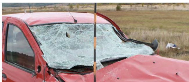
Fig. 2.23. Parbrizul deformat spre interior
