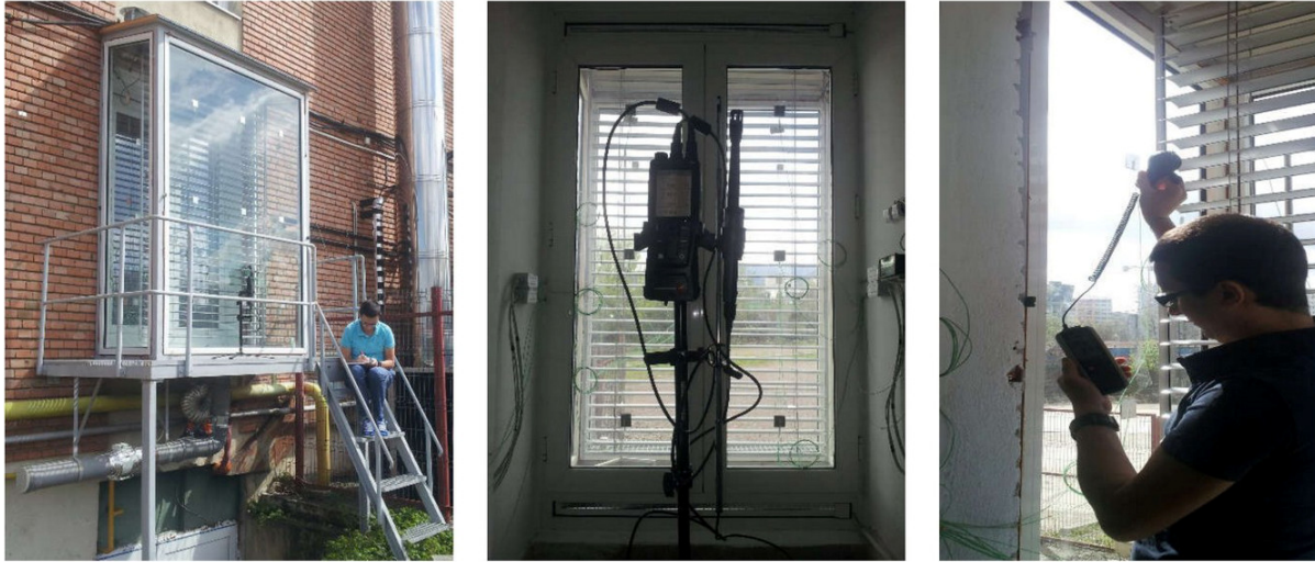
Figure 76. Box window double-skin façade laboratory
