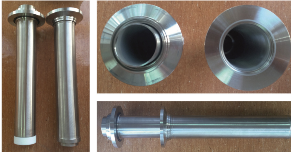
Figure 41. Vacuum insulated pipe element for cryogenic fluid transport
