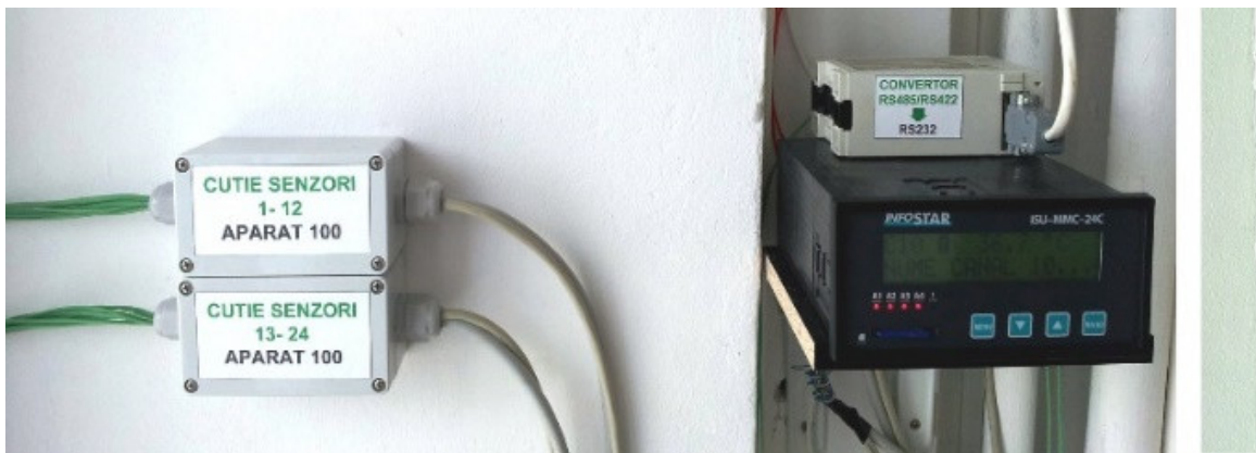
Figure 21 . ISU-MMC-24C, the converter RS485/RS422-RS232 and cases related to the 24 temperature sensors
