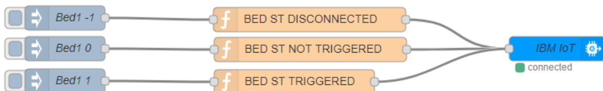
Figure 59 - Sensor status testing flow
