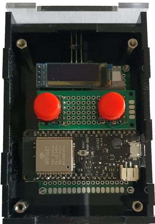
Figure 28 - The electronic of the SAVE Sensors Adapter
