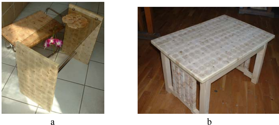
Figure 68 Panels with crosscut grain made of branch wood and their possible use in small furniture objects (Gurau et al. 2008b)
