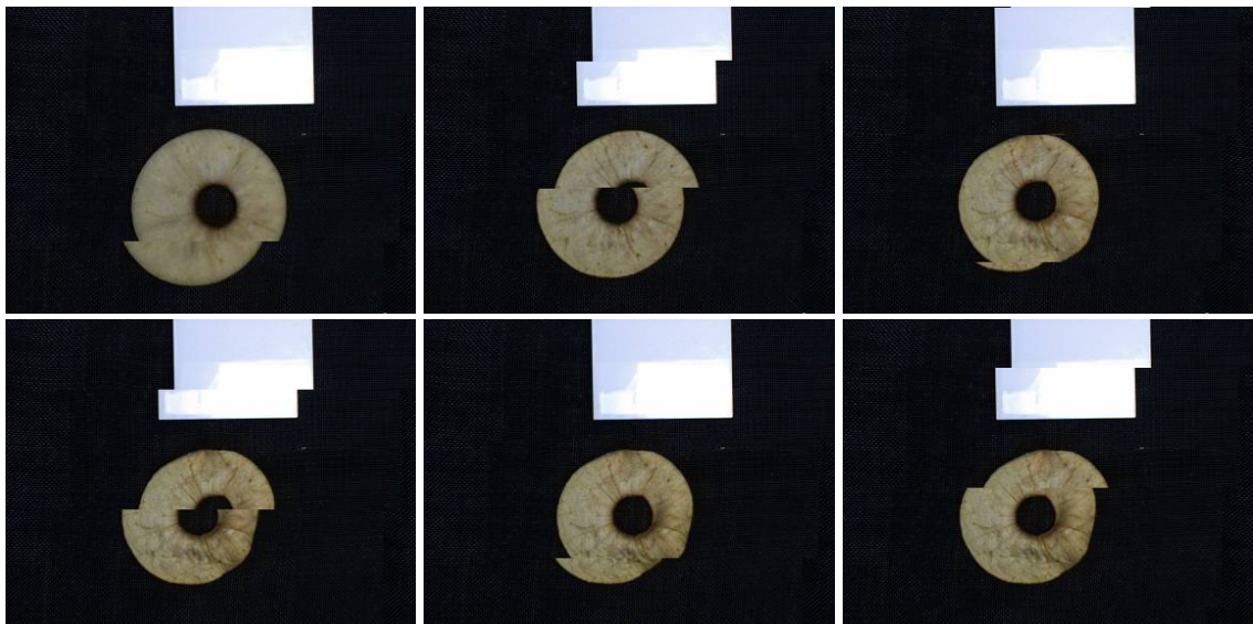
Figure 3.4. Images of apple slices during drying process (intervals 40 min, drying agent temperature= 60 °C) (apple, Golden Delicious variety)
