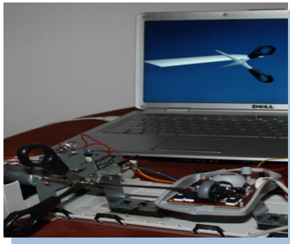
Fig.2.2.6 Scissors device (bottom- side of the picture) and virtual scissors prototype (up- side of the picture)
