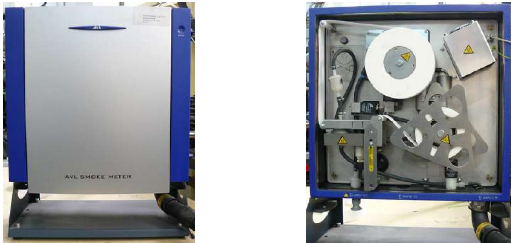
Fig.1.30 AVL 415S Smoke meter
