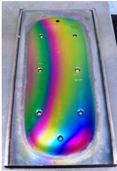
Fig. 1.3 The erosion track on a rectangular titanium target with gold spots.
