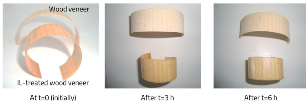
Figure 2.13. Photographic images illustrating the plasticization of wood by HMIMCl (POSDRU/89/1.5/S/59323 postdoctoral experimental report, 2011)
