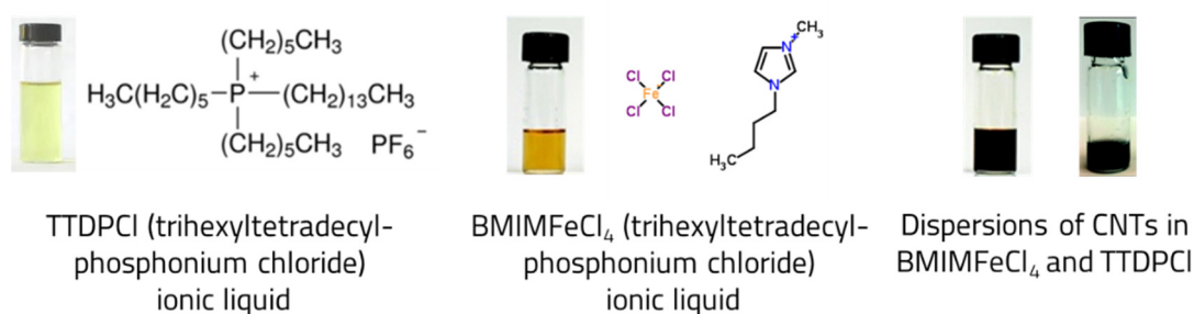
Figure 3.17. Photographic images of the ILs, of the resulted MWCNTs/IL dispersions and the structural formulas of the phosphonium and imidazolium ILs (unpublished results, PNII-RU-TE-2014-4-0173 final synthetic report, 2017 )
