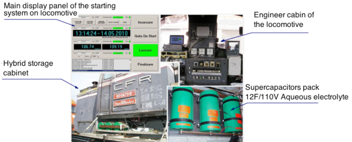
Figure 20. Pictures with some details of starting-system implementation on LDH1250HP shunting locomotive
