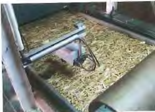
Oriented strands in crosswise direction
