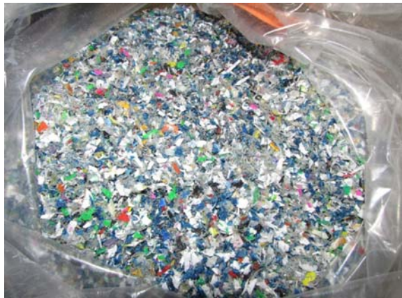
Figure 2.1. Cut polymeric wastes selected by Urban Company, from MSW of Brasov, Romania prepared for separation process (W2Plastics/D4.1) [16]
