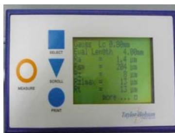
Figure 4.5. The parameters tested with Surtronic 25 [100]
