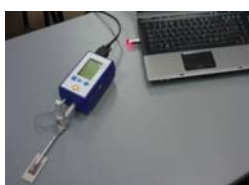
Figure 4. 4. Calibration of the roughness checker [100]
